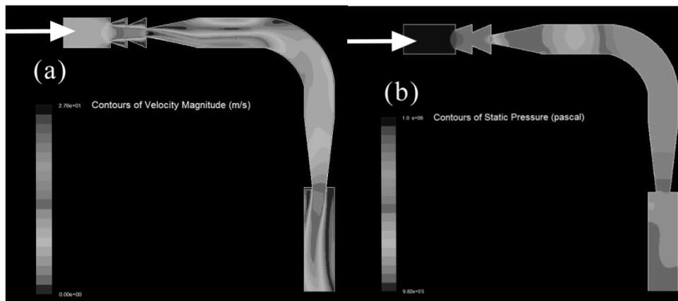
Figure 3. Contours of velocity and pressure inside of the protected bend
