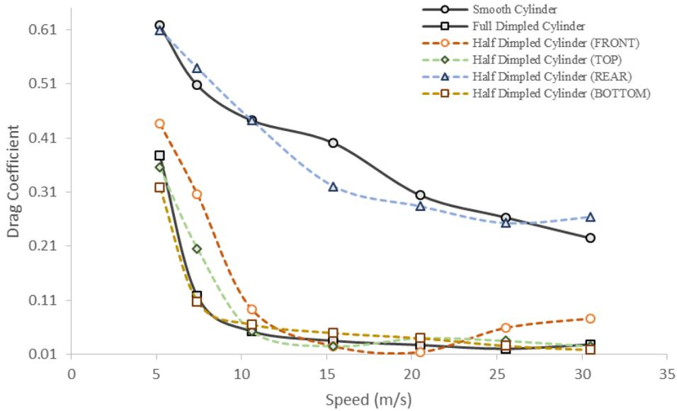
**Fig. 3.** Graph of Drag Coefficient against speed for all types of cylinders
