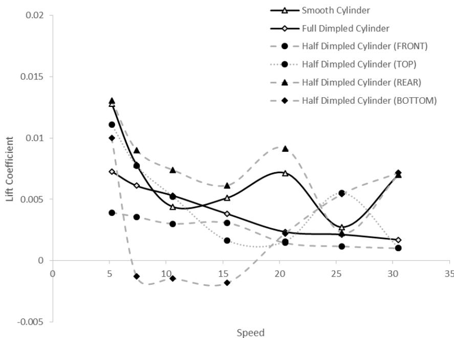
**Fig. 4.** Graph of Lift Coefficient against Speed for all types of cylinders
