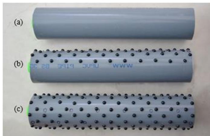
**Fig. 2.** Final product for test object which is smooth cylinder (a), outward dimple on half surface (b) and outward dimple on full surface (c)
