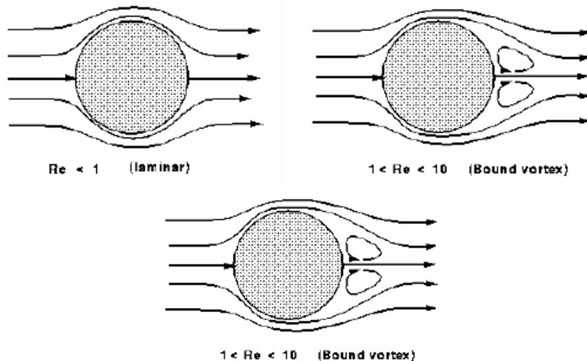
**Fig. 1.** Reynolds number on flow pass a cylinder [16]
