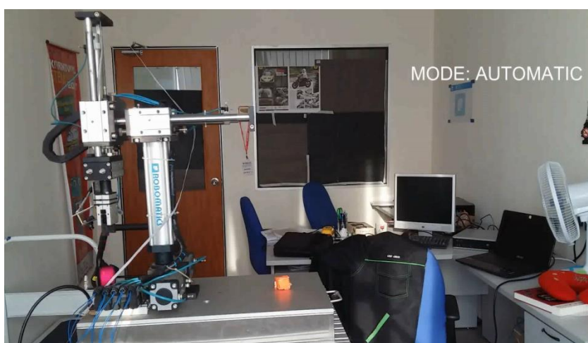
(c) gripper transfer the object to another designated position and release it
