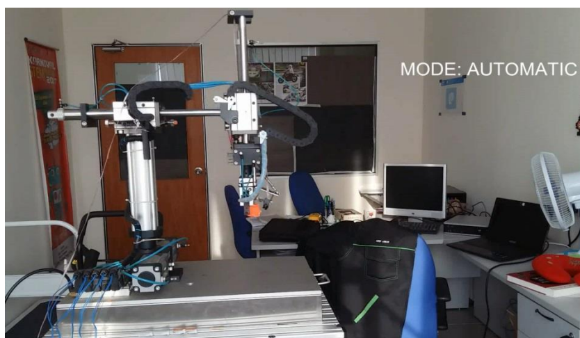
(c) object is raised, transferred horizontally to a designated receiving point
