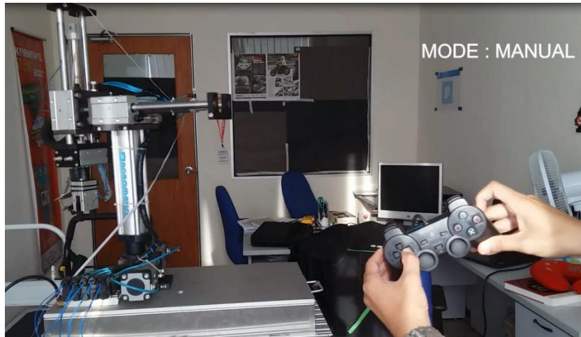
(e) pick and place robot rotates 180° anti-clockwise by pushing button ►
