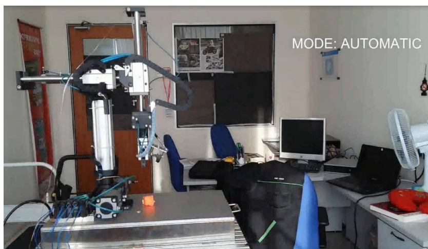
(a) gripper moves downward to grasp the orange object at the designated starting point
