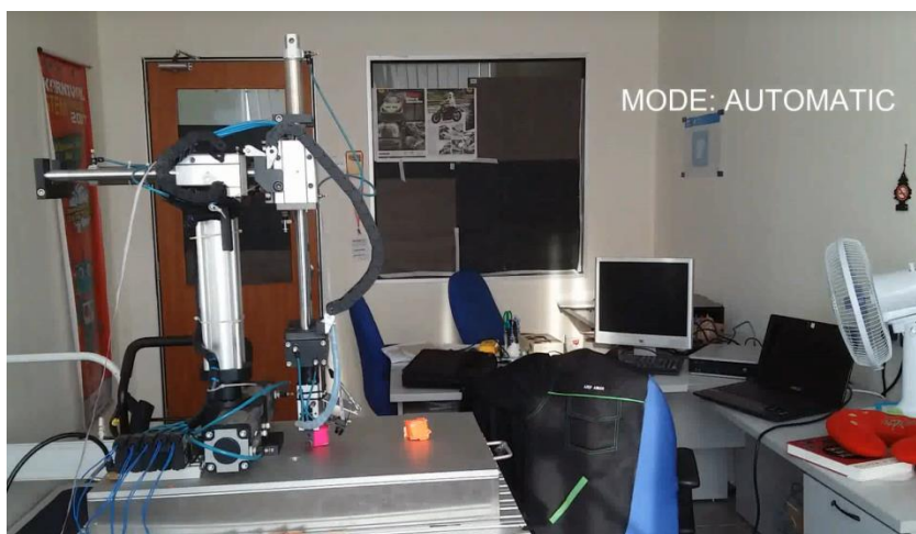
(a) gripper grasps the red object at the designated starting point
