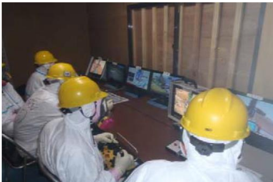
Fig. 1. Interface for nuclear disaster teleoperation. Note the use of gas mask on the teleoperator
