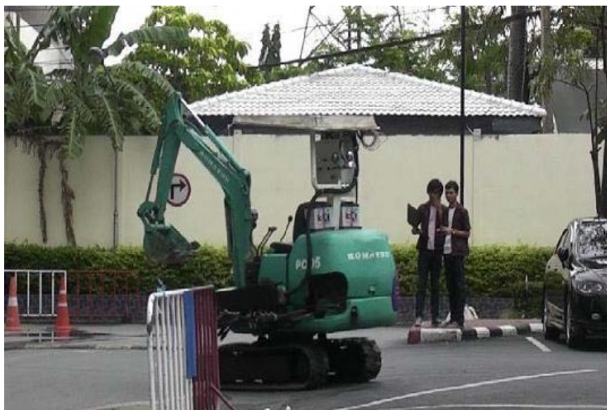
Fig. 13. Teleoperated excavator from King Mongkut's University of Technology
