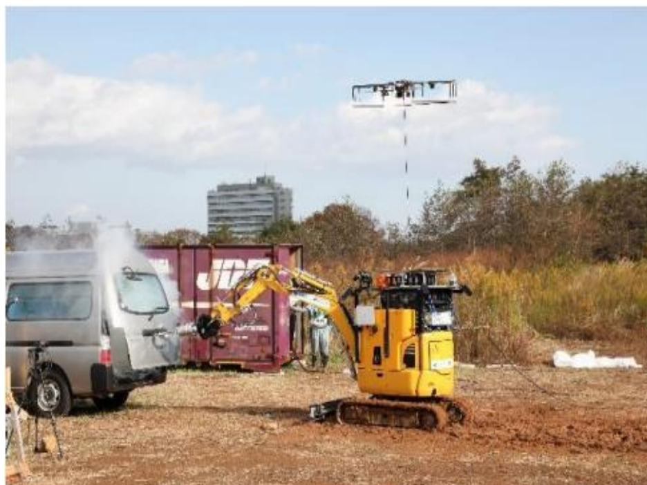
Fig. 26. Field test of the excavator with drone support
