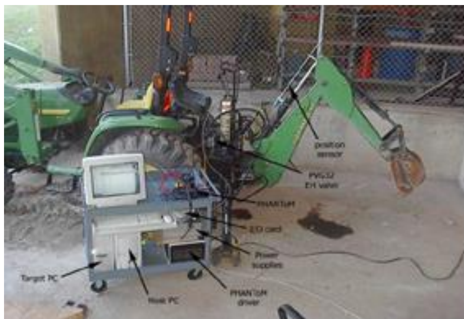
Fig. 6. Haptic small backhoe
