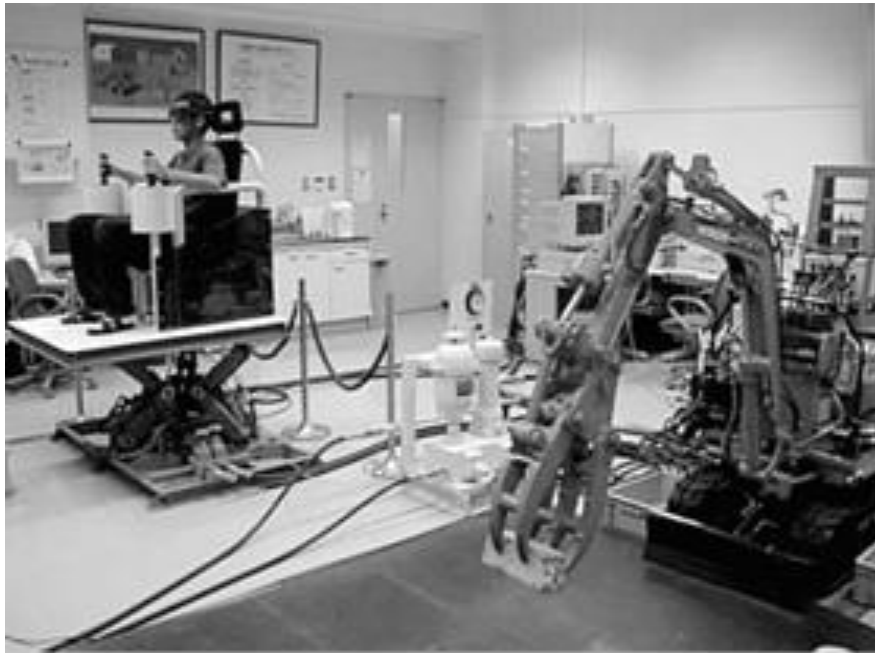
Fig. 12. Teleoperated excavator with tele-grasping performance at Gifu University
