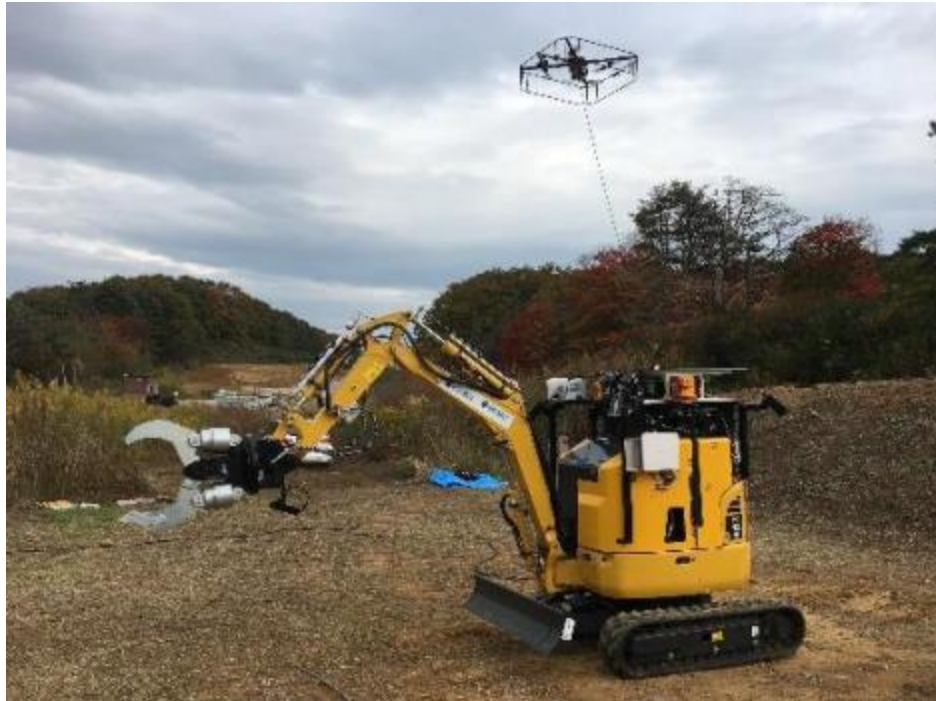
Fig. 25. Teleoperated excavator with drone support
