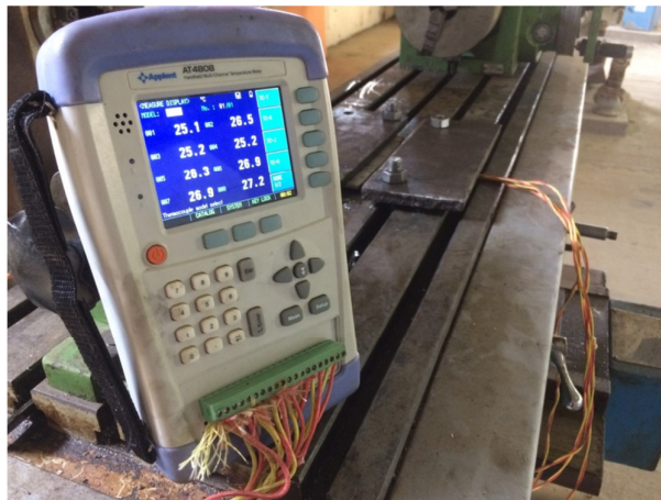
Fig. 5. The data logger used in measuring temperature
