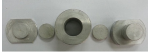
Figure 1: Aluminium mould used to produce sample.
