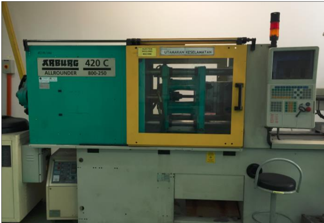
Fig. 2. Injection molding machine used in the experimental work
