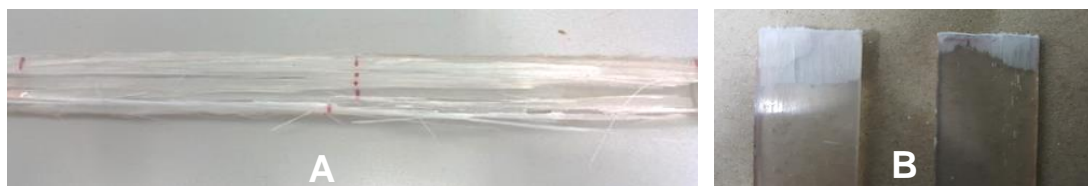
Fig. 2. (A) Fractured Test Specimen from Preliminary Tensile Test, (B) Fractured Test Specimen After an Incision Was Introduced
