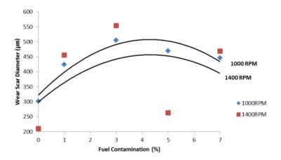
**Figure 6:** Graph of wear scar diameter  $[\mu m]$  against fuel contamination [%]
