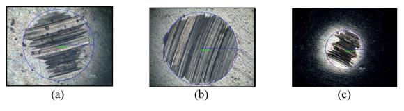
**Figure 8:** (a) Worn surface at 1000 RPM, 1% contamination; (b) Worn surface at 1400 RPM, 1% contamination; (c) Worn surface at 1000 RPM, 7% contamination
