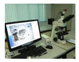
Figure 3: High resolution computerized microscope Motic BA310MET
