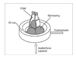
Figure 2: Schematic diagram of the Four Ball Tribotester assembly [5].
