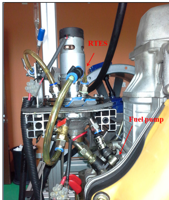
Figure 3: Location of RTES during the engine test
