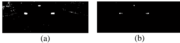
Fig. 8. Sample image in binary image (a) before morphology operation (b) after morphology operation
